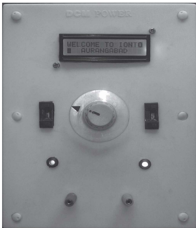
Fig.2 Iontophoresis Power supply and Data Acquisition System.
